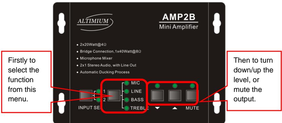
For example, to turn up the line volume, you should select the "LINE" first, and then press the button "▲".
